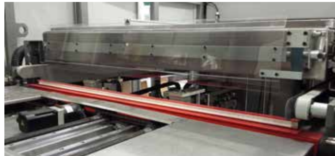
Sheet cleaning system with ionized air: eliminates electrostatic charges from each sheet and from the pallet installed in the loading zone. The utmost in terms of thermoforming quality and safety.
