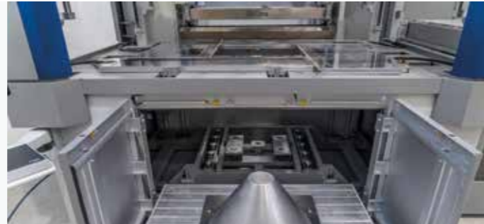
Quick mould change: removable mould plate with its own cart. The cart can be fitted with mould lifting device for the utmost in terms of production change speed. Simplifies the centring operations and equipment installation on the outside of the machine.
